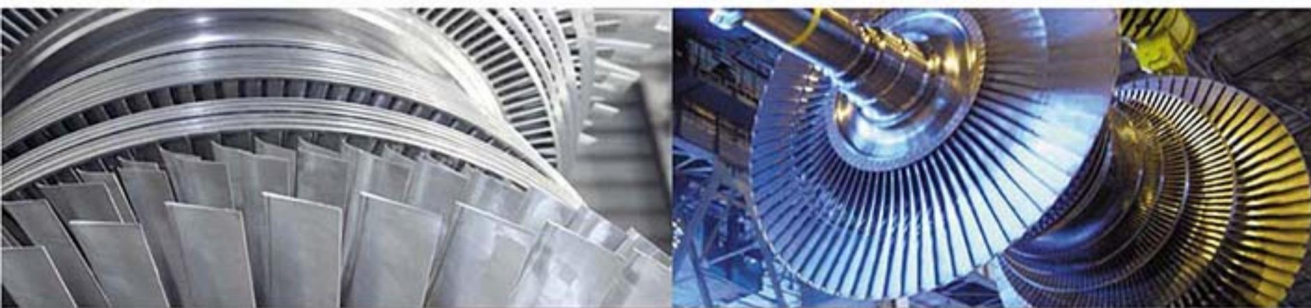
The training covers the turbine and turbine auxiliaries. The turbine is nothing more than a heat machine. It converts the heat energy in the steam to mechanical horsepower to drive the generator. The generator, of course, changes mechanical energy to electrical energy.
